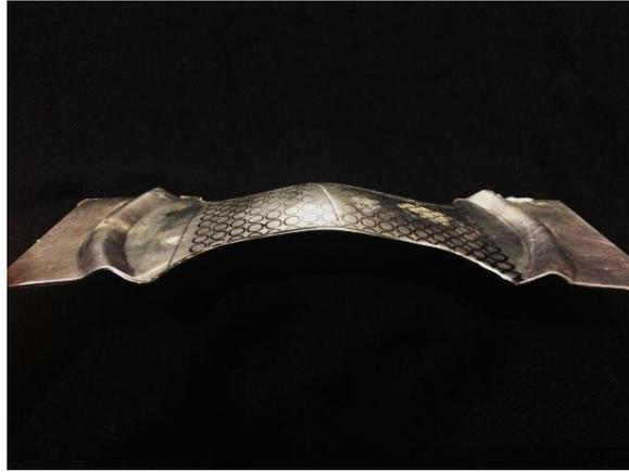
Fig. 4. The 75 mm×200 mm specimen after forming.
