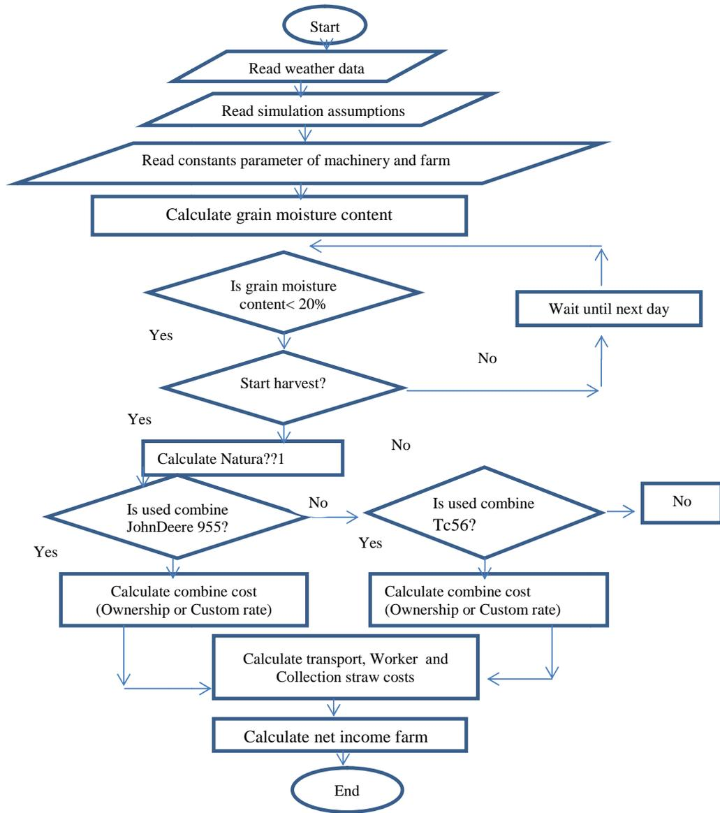
Fig. 1. Flowchart of the Wheat Harvest Simulation Model
