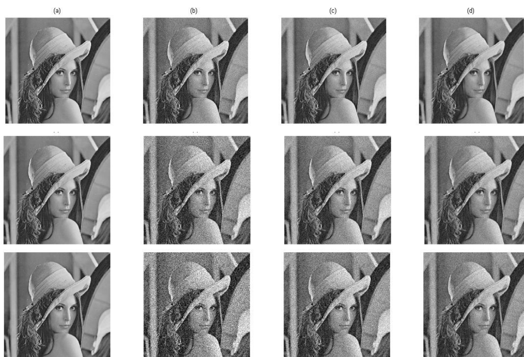
Fig. 3. Experiment for "Lena". (a) original image. (b) corrupted image by Gaussian noise for \sigma=10, 20 and 30 . (c) Gaussian smoothing filter. (d) FCE proposed filter
