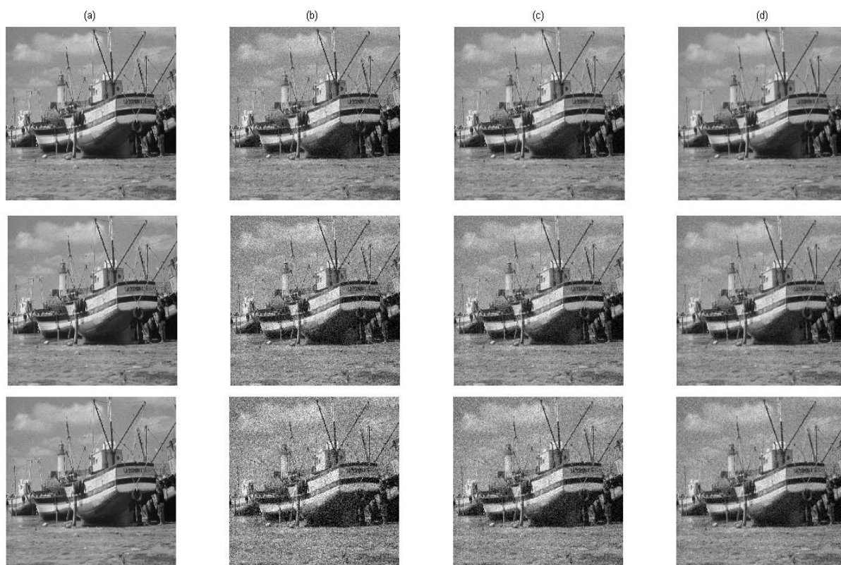
Fig. 5. Experiment for "Boat". (a) original image. (b) corrupted image by Gaussian noise for \sigma=10, 20 and 30 . (c) Gaussian smoothing filter. (d) FCE proposed filter
