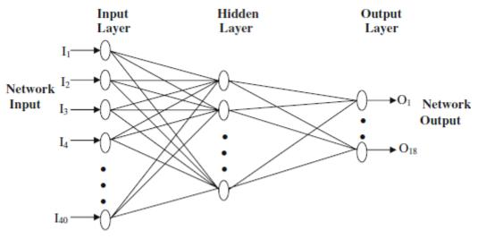
Fig. 3. Three-layer LMBP neural network architecture
