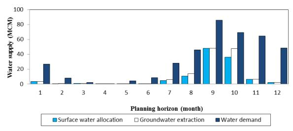
Fig. 7. The water demand and monthly allocated surface water and groundwater to Nekouabad left zone
