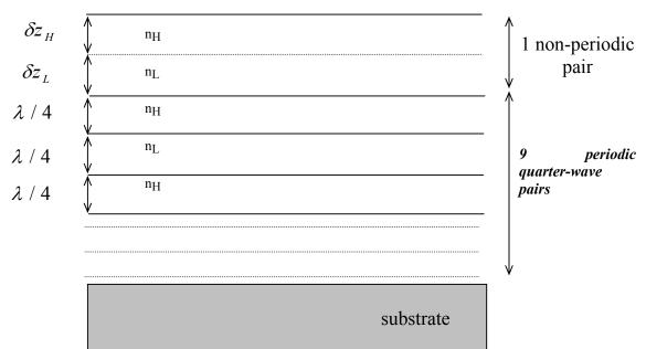
Fig. 1. Schematic diagram of a typical 10 pairs (1 non-periodic and 9 periodic pairs) multi-layer mirror
