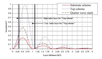
Fig. 2. The electric field distribution within the optical layers for normal incidence, using: "quarter- wave stack", "top scheme", and "substrate scheme"
