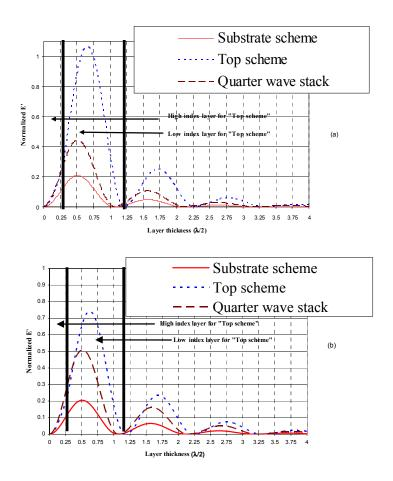
Fig. 3. The electric field within the optical layers for a laser beam with an incident angle of 40° with: (a) polarization S, and (b) polarization P
