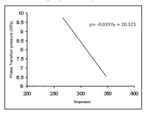
Fig. 4. Variation of phase transformation pressure (Pt) with temperature in P-type silicon
