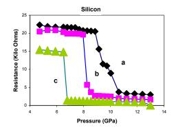
Fig. 2. Variation of electric resistance of P-type silicon Vs. pressure at different sample temperatures: a)-5 °C ,b)20 °C, c)60 °C *Iranian Journal of Science & Technology, Trans. A Volume 30, Number A3*
