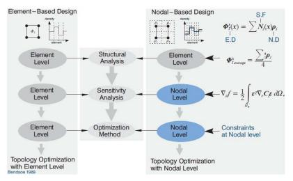
Fig. 5. Algorithm comparisons of element- and node-based design in material topology optimization
