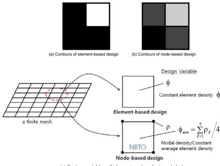
(c) Design variables of element and node-based design
