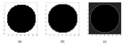
Fig. 8. Material layouts of a circle: (a) element-based design, (b) node-based design, (c) 0.5 isoline layout of node-based design
