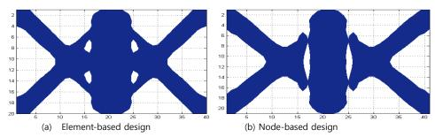
Fig. 14. Optimal topologies for dynamic topology optimization design under material volume 50%: 0.5 isolines
