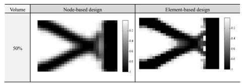
Fig. 10. Optimal topologies for dynamic topology optimization design: density distribution contours
