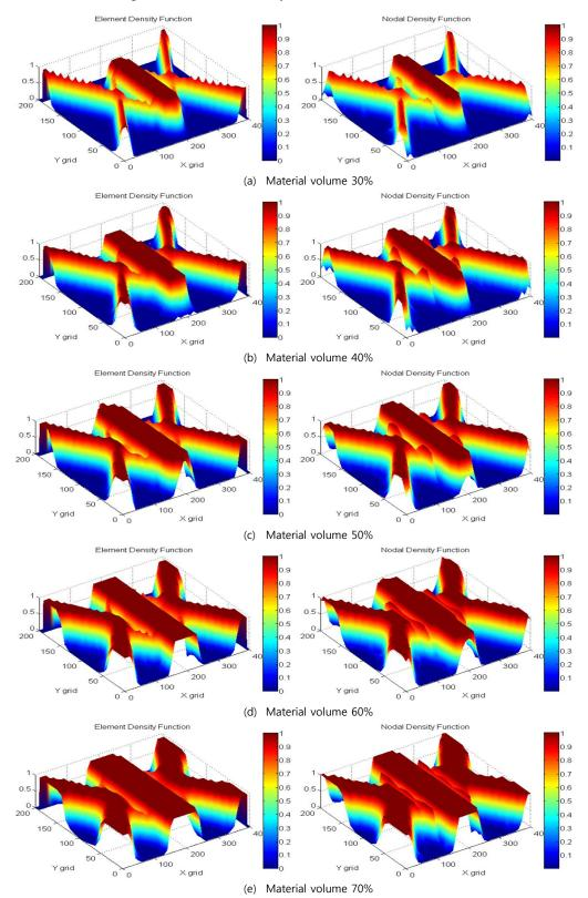
Fig. 15. Optimal topologies for dynamic topology optimization design: three-dimensional density function
