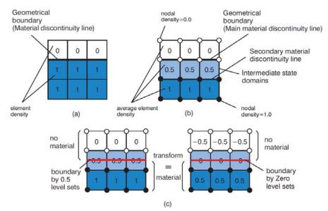
Fig. 7. Representations of material layouts of element- and node-based design: (a) element-based design, (b) nodebased design, (c) the use of zero or 0.5 isoline (level sets) for describing material layouts Analysis models
