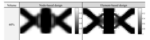
Fig. 13. Optimal topologies for dynamic topology optimization design: density distribution contours
