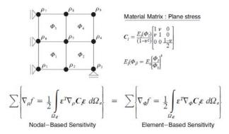
Fig. 6. Duality of sensitivity analysis in element- and node-based design in material topology optimization
