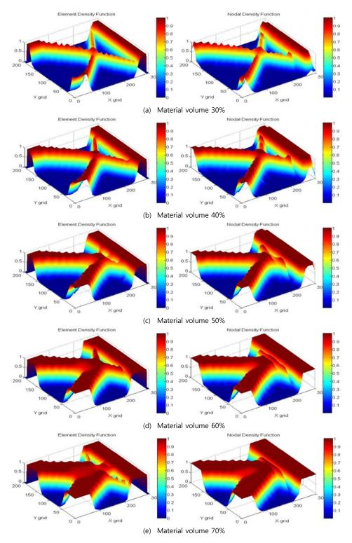
Fig. 12. Optimal topologies for dynamic topology optimization design: three-dimensional density function
