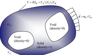
Fig. 1. Schematic for the material topology optimization of continuous structures
