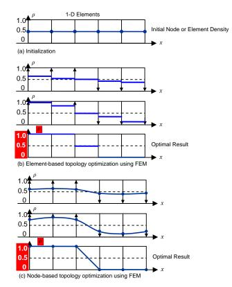
Fig. 4. Element- and node-based topology optimization processes in a given volume constraint of 50%
