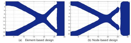
Fig. 11. Optimal topologies for dynamic topology optimization design under material volume 40%: 0.5 isolines
