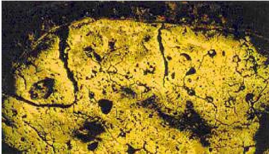
Fig. 19. Simple massive pisoid lag, in which the massive maghemite core contains prominent radial cracks (field of view is 3.5 mm)
