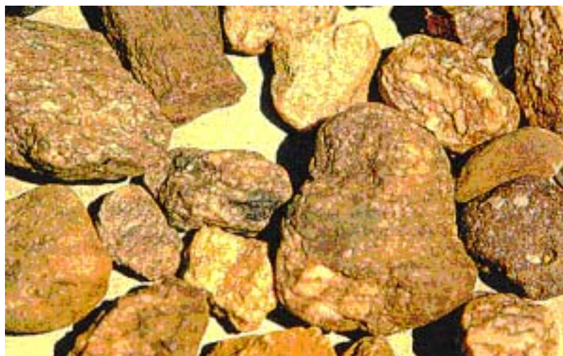
Fig. 23. Moderately rounded silcrete lags with smooth cusped surface and brecciate fabrics in some lags (field of view is 10 cm)
