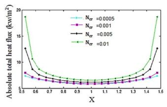
Fig.12. The effect of Conduction-radiation parameter on the absolute total heat flux over the bottom wall, for ( $\lambda = 0.00044$ ,  $\varepsilon_w = 1.0$ ,  $\beta = 1.0$ ,  $\omega=0.5$ )
