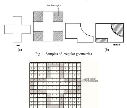
Fig. 2. A domain with blocked-off/inactive region
