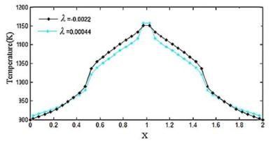
Fig. 8. Temperature distribution in the section AA', for two different values of  $\lambda$ , (N<sub>cr</sub> = 0.00033,  $\varepsilon_w = 1.0, \beta = 1.0, \omega = 0.5$ )
