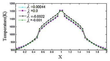
Fig. 7. The effect of conductivity-temperature coefficient on the distribution temperature in the section AA', for (N<sub>cr</sub> = 0.00033,  $\varepsilon_w = 1.0$ ,  $\beta = 1.0$ ,  $\omega=0.5$ )
