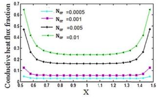
Fig.11.The effect of Conduction-radiation parameter on the conductive heat flux fraction over the bottom wall, for ( $\lambda = 0.00044$ ,  $\varepsilon_w = 1.0$ ,  $\beta = 1.0$ ,  $\omega=0.5$ )
