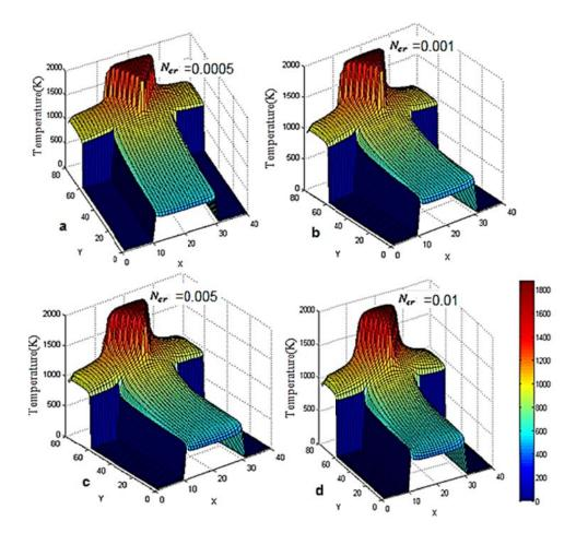
Fig. 13. The effect of Conduction-radiation parameter on the temperature distribution within enclosure. (a):N<sub>cr</sub>=0.0005,(b):N<sub>cr</sub>=0.001, (c):N<sub>cr</sub>=0.005,(d):N<sub>cr</sub> = 0.01, for ( $\lambda = 0.00044$ ,  $\varepsilon_w = 1.0$ ,  $\beta = 1.0$ ,  $\omega = 0.5$ )
