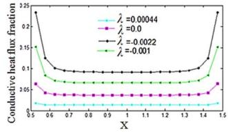
Fig. 10. The effect of conductivity-temperature coefficient on the conductive heat flux fraction over the bottom wall, for ( $N_{cr} = 0.00033$ ,  $\varepsilon_w = 1.0$ ,  $\beta = 1.0$ ,  $\omega=0.5$ )
