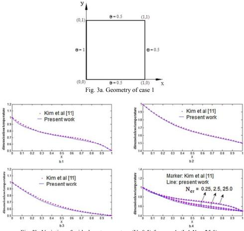
Fig. 3b. Variation of mid-plane temperature (Y=0.5) for case 1; (b.1: $N_{cr}$ =25.0), (b.2:  $N_{cr}$ =2.5),(b.3:  $N_{cr}$ =0.25),(b.4: effect of  $N_{cr}$ ), comparison with the results of Kim et al [11]
