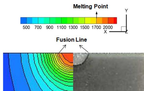
Fig. 7. Simulated and experimental weld pool obtained for sample 2, indicating a good agreement between the experimental and simulated data
