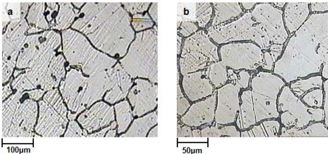
Fig. 8. Microscopic images taken from the sensitized zone in sample 2 at low (a) and high (b) magnifications. Formation of the chromium carbide along the austenite grain boundaries leads a chromium-depleted zone adjacent to the austenite grain boundary
