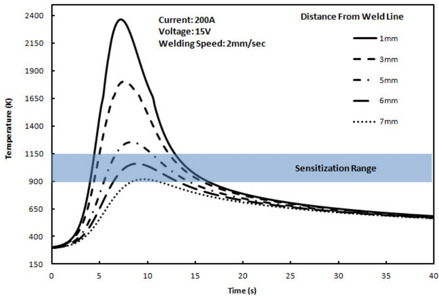
Fig. 3. Temperature variations at different locations from the weld line. The filled area shows the temperature range of sensitization (900 to 1150 K)
