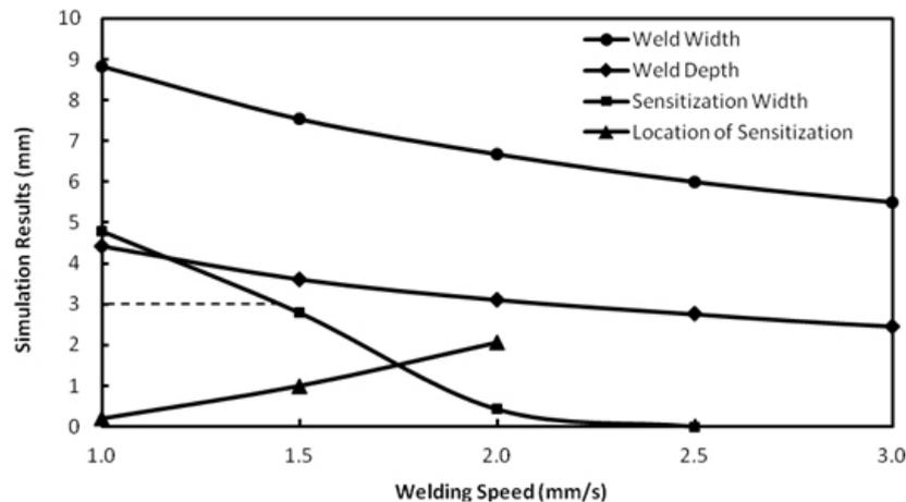
Fig. 6. Weld depth, weld width, sensitized size and its location from weld line as a function of welding speed. The sensitization size decreases and the sensitized location becomes farther from the weld line as the welding speed is increased
