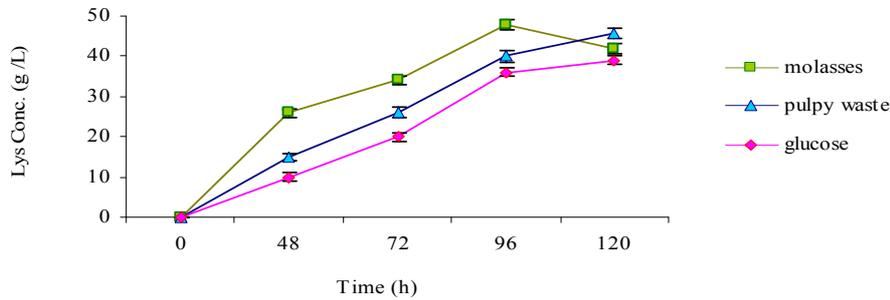
**Figure 3. Lysine concentration values versus time using different carbon sources**
