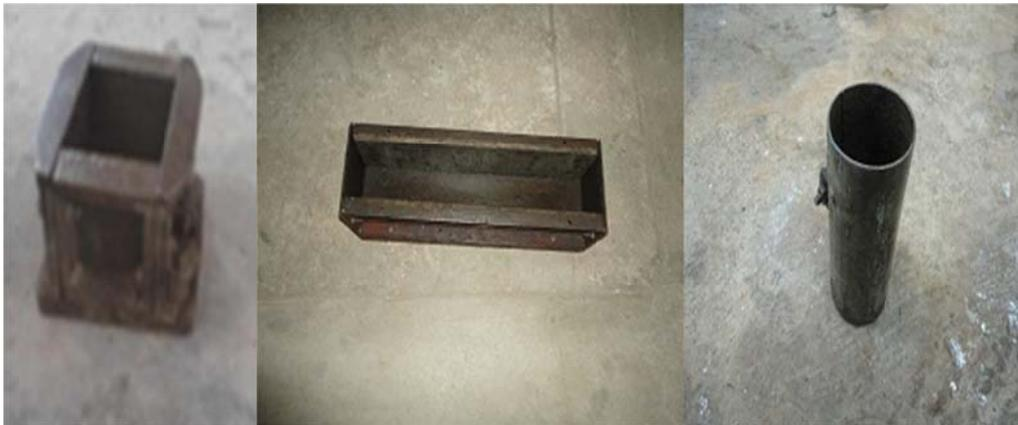
Fig. 7. Mortar mould for compressive strength, flexural strength and split tensile strength
