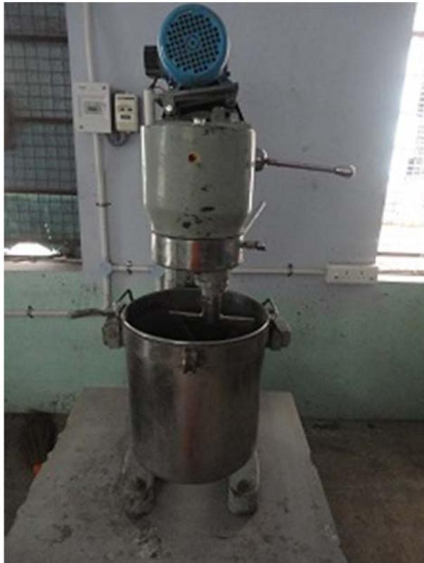
Fig. 4. Mixing of materials using Hobart mixer
