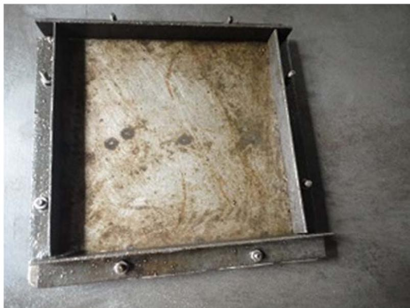
Fig. 5. Slab mould
