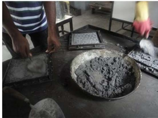
Fig. 6. Casting of geopolymer ferrocement slab specimen
