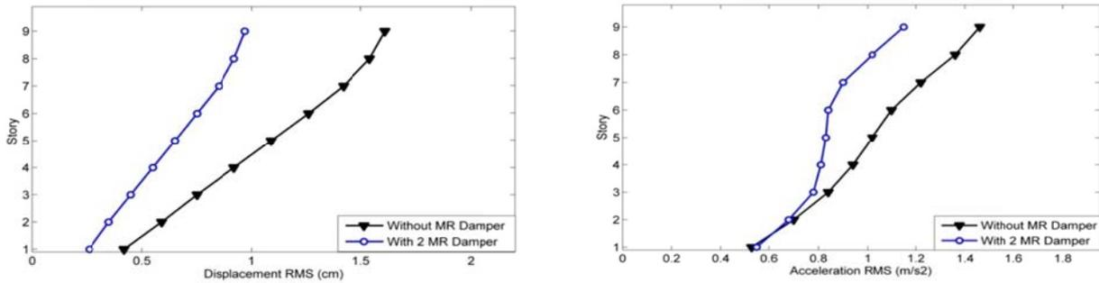
Fig. 11. Comparing RMS of displacement and absolute acceleration response in 9-story structure under the Kobe earthquake
