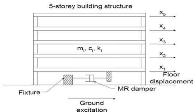
Fig 1. 5-Story steel frame model made in Technology University of Sydney [15]
