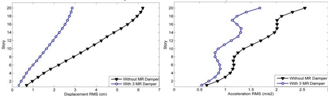
Fig. 14. Comparing RMS of displacement and absolute acceleration response in 20-story structure under the Northridge earthquake
