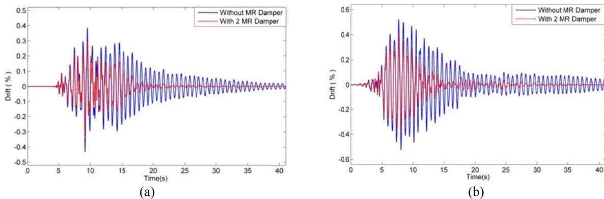
Fig. 7. Drift response of 9-story structure under a: the Kobe and b: the Northridge earthquake
