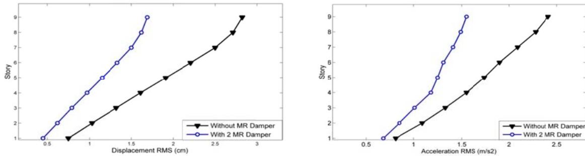
Fig. 12. Comparing RMS of displacement and absolute acceleration response in 9-story structure under the Northridge earthquake
