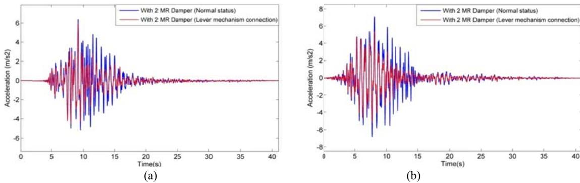
Fig. 21. Acceleration response of 9-story structure under a) the Kobe and b) the Northridge earthquake
