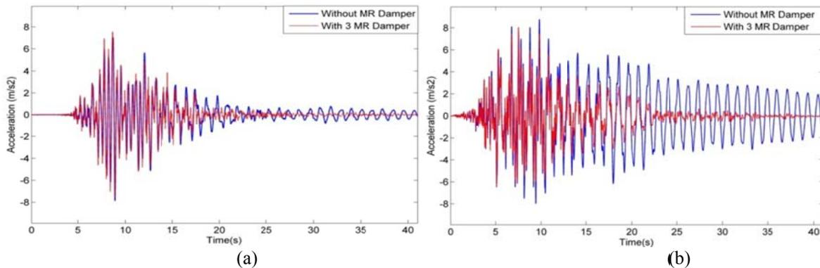
Fig. 10. Acceleration response of 20-story structure under a) the Kobe and b) the Northridge earthquake
