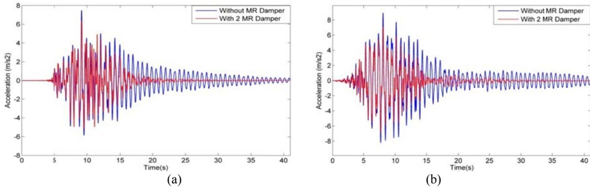
Fig. 9. Acceleration response of 9-story structure under a) the Kobe and b) the Northridge earthquake
