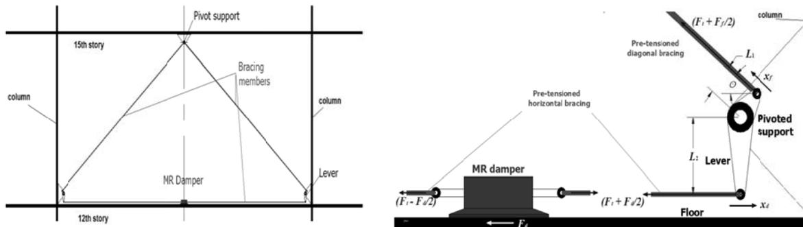
Fig. 17. MR damper between floor and lever mechanism connection [10]
