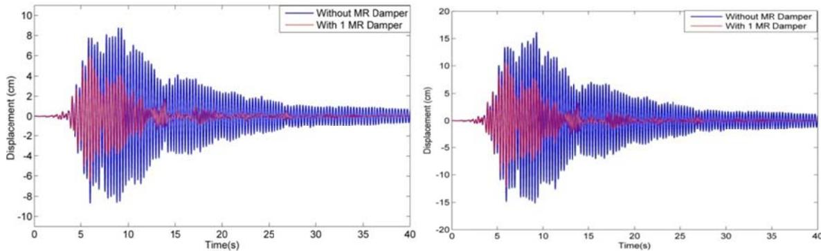
Fig. 2. Floor lateral displacement, 1<sup>st</sup> and 5<sup>th</sup> floors of 5-story steel frame model
