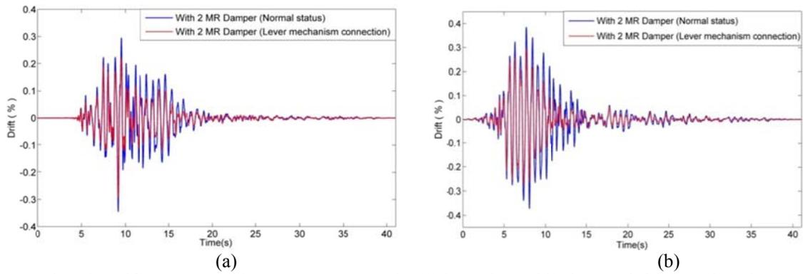
Fig. 19. Drift response of 9-story structure under a) the Kobe and b) the Northridge earthquake
