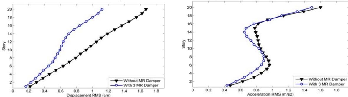
Figure 13: Comparing RMS of displacement and absolute acceleration response in 20-story structure under the Kobe earthquake
