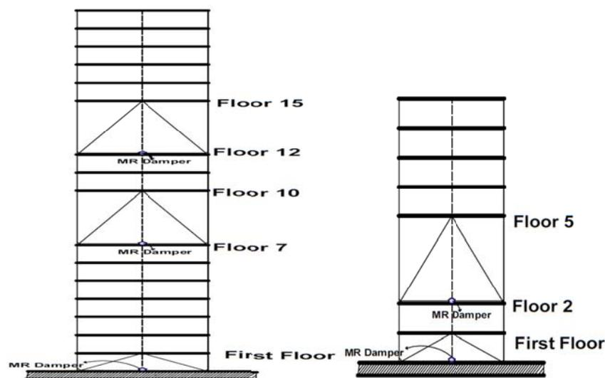
Fig. 18. Suggested positions for dampers placement
