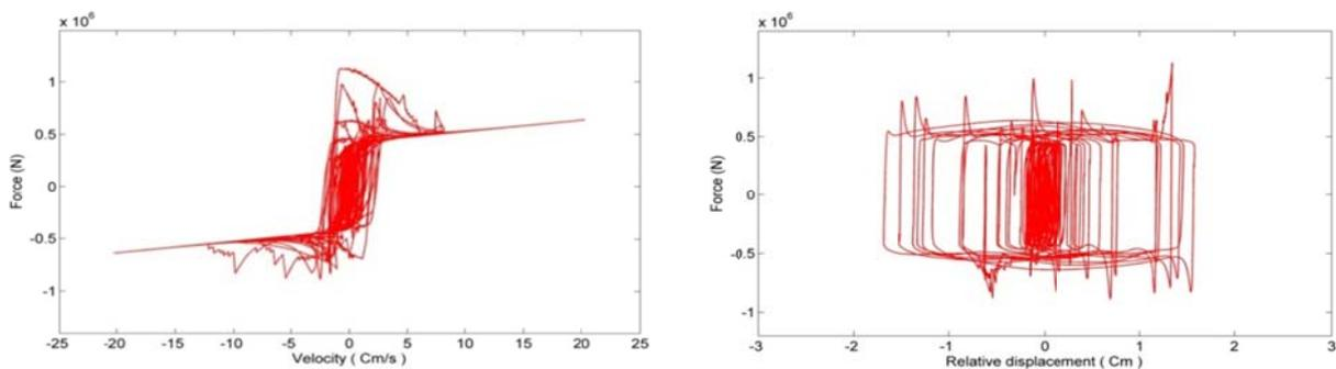
Fig. 15. Hysteretic curves of 9-story structure under the Northridge earthquake
