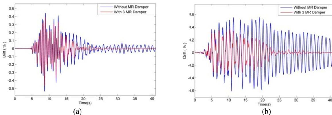
Fig. 8. Drift response of 20-story structure under a) the Kobe and b) the Northridge earthquake
