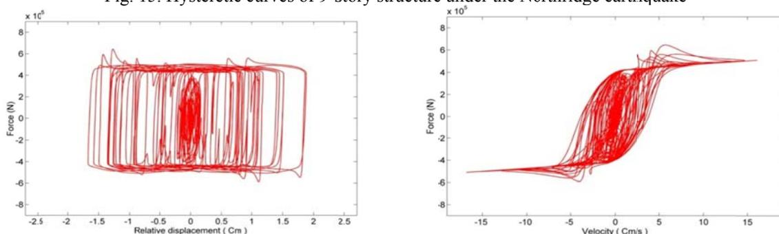
Fig. 16. Hysteretic curves of 20-story structure under the Northridge earthquake
