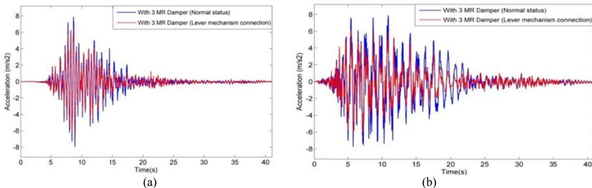
Fig. 22. Acceleration response of 20-story structure under a) the Kobe and b) the Northridge earthquake
