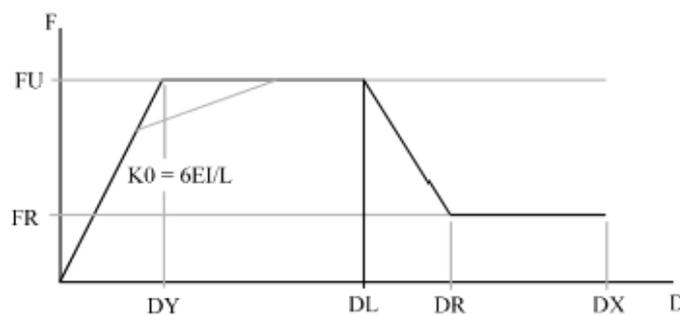
Fig. 5. Force-deformation relationship [39]
