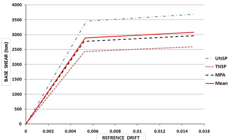
Fig. 9. The ideal bilinear diagrams of the pushover analyses for model A
