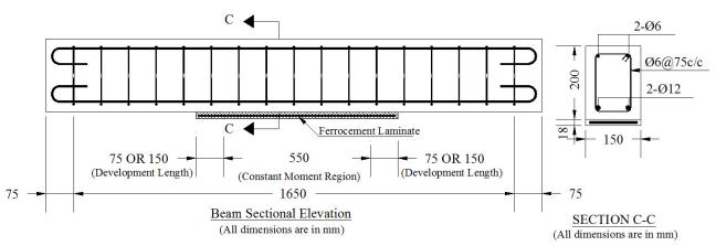
Fig. 7. Detail of beam with precast Ferrocement Laminate B (Group 'C')
