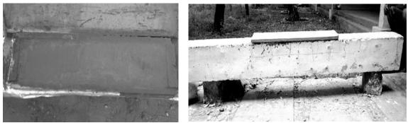
Preparation of Ferrocement Laminate Ferrocement Laminate placed to the inverted beam Fig. 8. Inverted beam with precast Ferrocement Laminate *B* (Group 'C')
