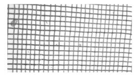
Fig. 1. Sample woven Ferro-mesh
