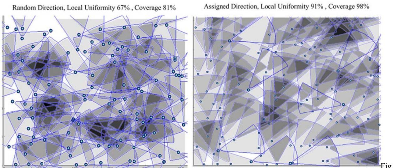
7. Sensor assignment to region. (a) The initial direction of sensors is random.
