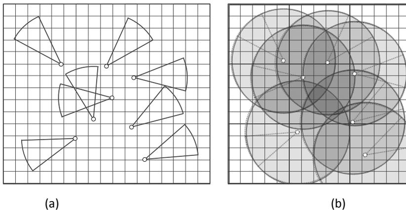
Fig. 4. The area covered by sensors to measure the areas energy. (a) Directional sensing area, (b) Omni-directional sensing area (or potential coverage area of the directional sensor with rotational capability)
