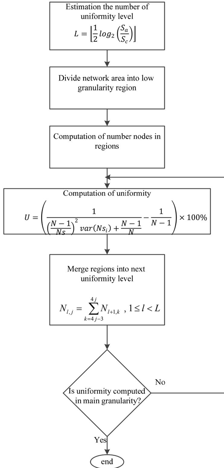
Fig. 3. Uniformity calculation flowchart
