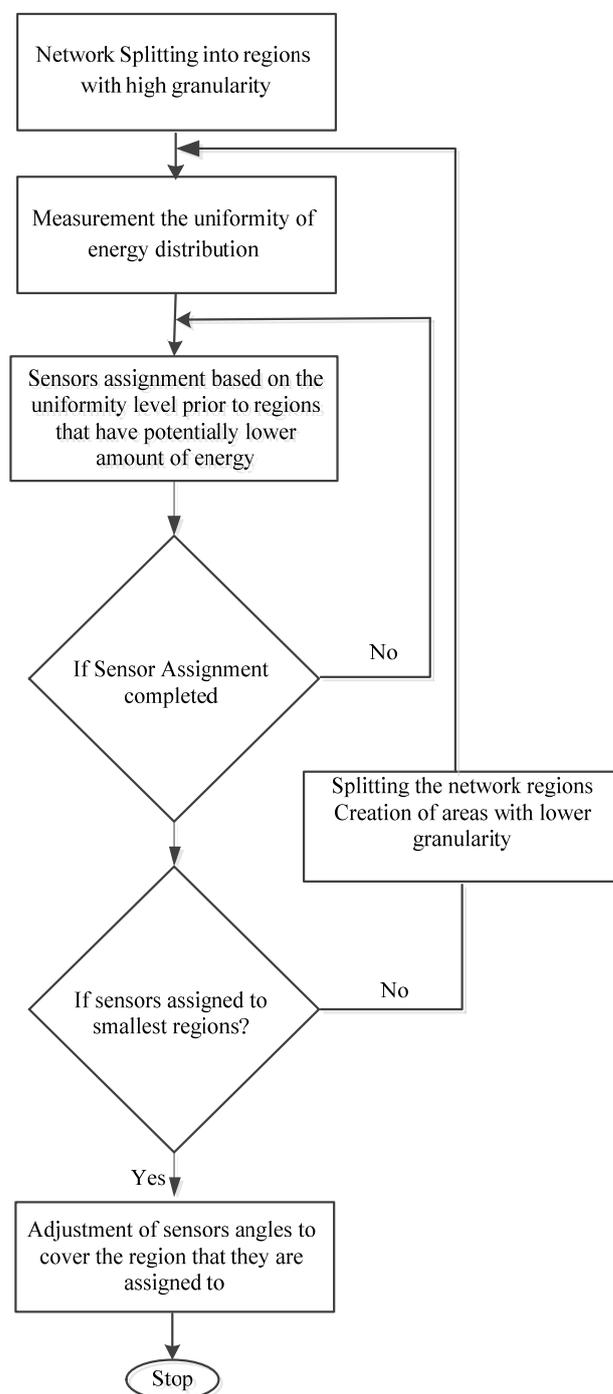
Fig. 6. Algorithm flowchart of sensor assignment to the network regions
