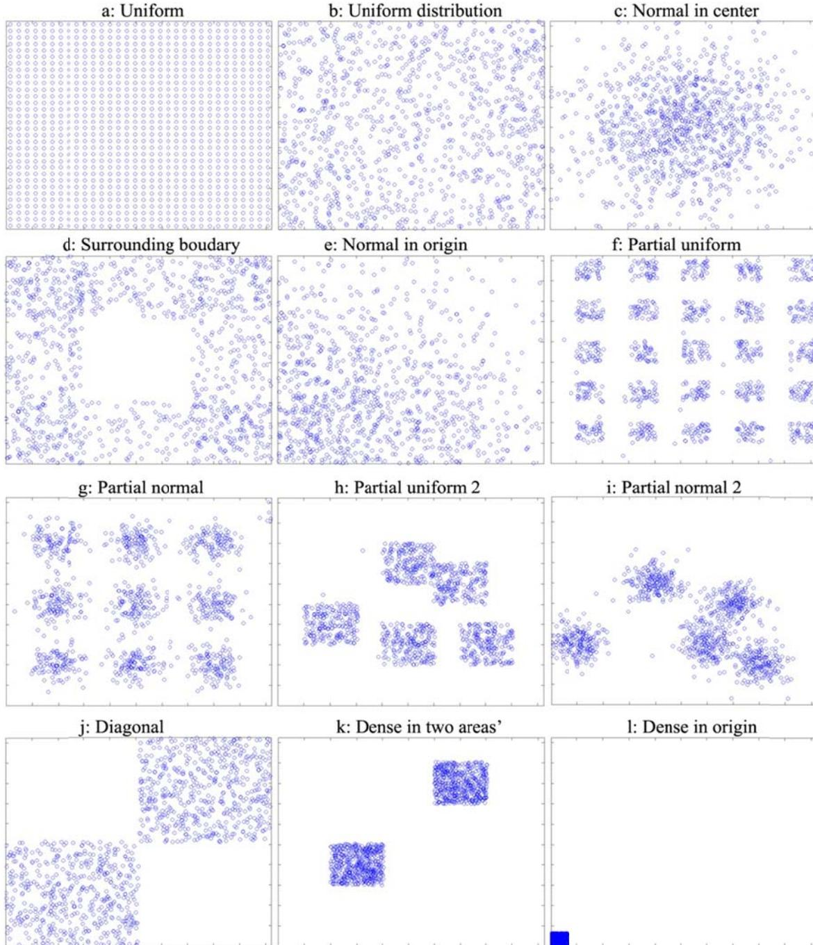
Fig. 10. A set of sensor distribution trial patterns in the network [22]
