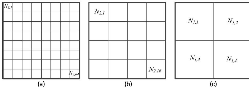
Fig. 1. The network regions classification in three levels: (a) low granularity regions for local uniformity measurement, (b) medium granularity, (c) high granularity regions for the global uniformity measurement
