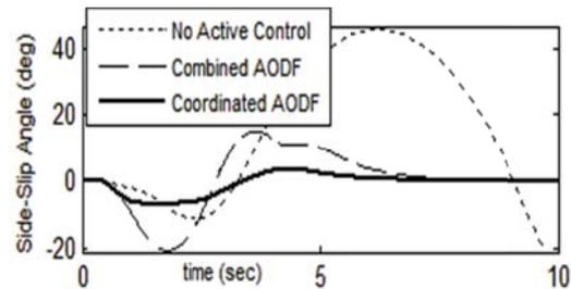
Fig. 16. Side-slip angle in SLC with driver's braking
