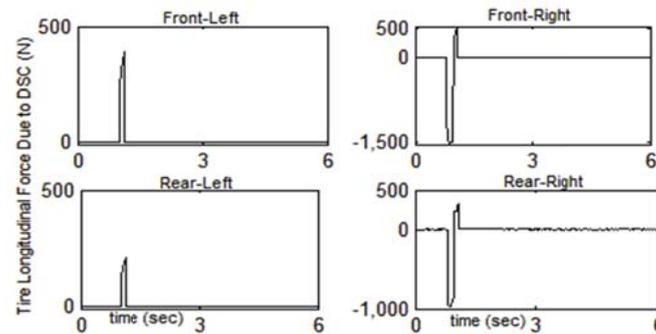
Fig. 18. Longitudinal forces by DSC in SLC with driver's braking
