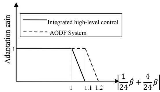
Fig. 5. Adaptation gains in different phases of IVDC
