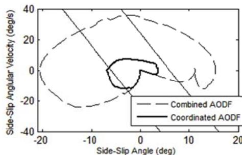
Fig. 17. Phase-plane trajectory in SLC with driver's braking
