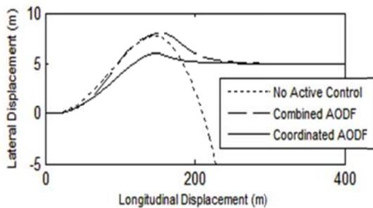
Fig. 14. Vehicle path in SLC with driver's braking
