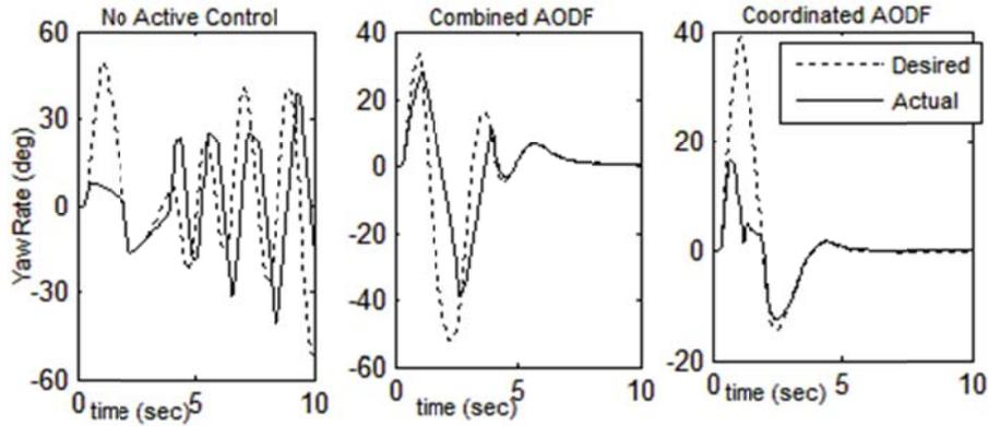
Fig. 8. Yaw rate in SLC without driver's braking
