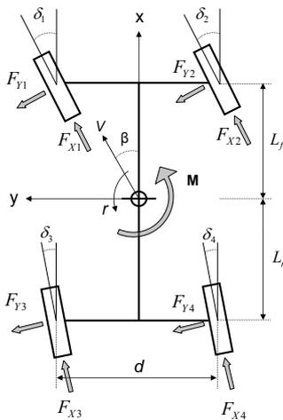
Fig. 4. Vehicle dynamics model schematic in top view
