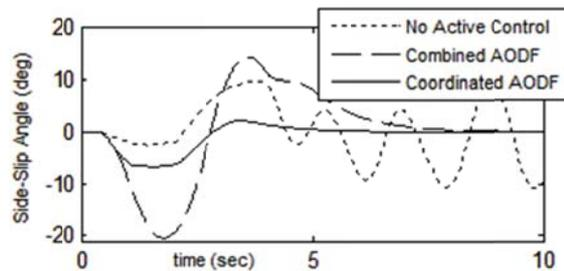
Fig. 9. Side-slip angle in SLC without driver's braking
