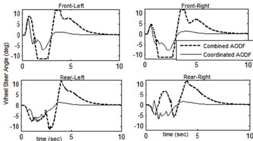
Fig. 13. Active steering in SLC without driver's braking
