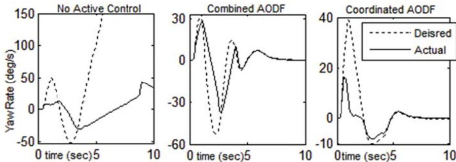
Fig. 15. Yaw rate in SLC with driver's braking
